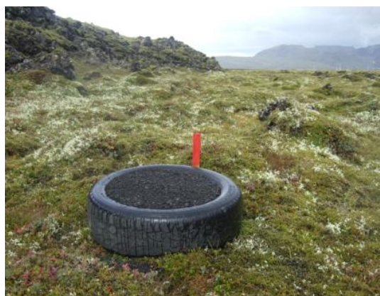
Figure 5 – A fixed monitoring site for CO 2 flux measurements. Photo: Hólmfríður Sigurðardóttir
